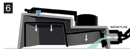
Once the water/nutrient solution drops below the Main Body of the AQUAvalve the surface tension around the AQUAvalve Main Body will break, this can take up to an hour. The vacuum in the Main Body is then released and the Inner Float drops to a position where the inlet can reopen and the filling process begins again.
