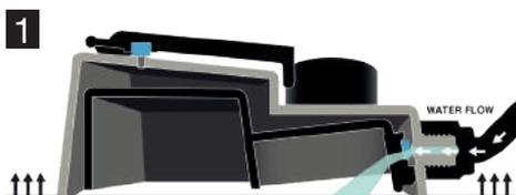
Once the AQUAvalve is positioned in a tray and connected to the water supply and the supply is turned on, water will begin to flow into the tray through the AQUAvalve nozzle. The Inner Float will rise a little but the Top Float will remain in position, keeping the hole sealed on the Main Body and preventing the Inner Float from rising further.
