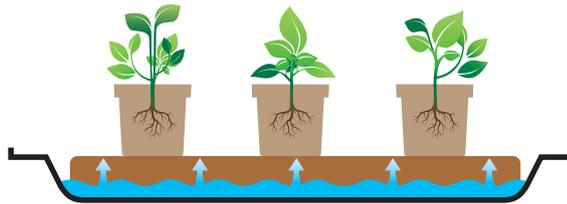
The CocoMat controls watering by holding and gradually wicking the water to the plants via capillary action.
