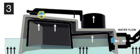
Once the water reaches 20mm / 1" (half way on the AQUAvalve collar) the Top Float will lift allowing the trapped air inside the Main Body to escape and simultaneously the Inner Float will rise and cut off the incoming water.
