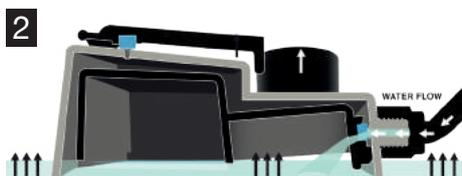
Trapped air inside the Main Body is unable to escape as the silicone in the Top Float is creating a seal on the Main Body, water continues to enter into the tray as the Inner Float is unable to shut off due to the trapped air.
