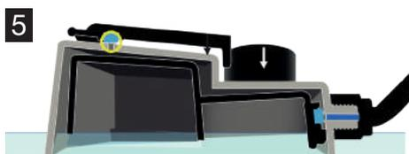
The sealing of the Main Body ensures that there is an air tight seal which in turn creates a vacuum inside the Main Body, this prevents the Inner Float from dropping and preventing any further water/nutrient solution from entering.
