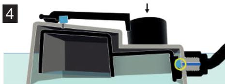
As the plants consume the nutrient solution the Top Float begins to drop back down re-sealing the hole on the Main Body creating an air tight seal.
